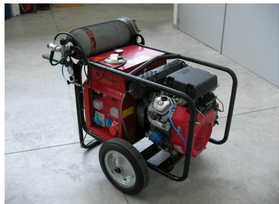
**Fig 1.** Photograph of the completely modified generator showing the gas cylinder used to store the hydrogen fuel.
